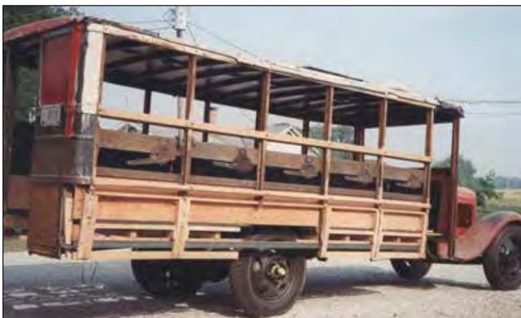
The body sports a new wood frame, ready for new sheet metal siding.
