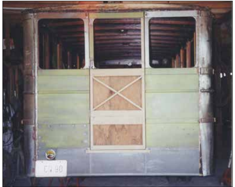
The center panel in place in the back door
