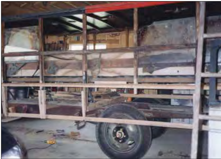
The bus body after sheet metal was stripped off
