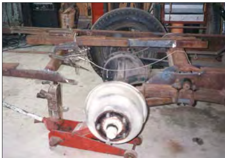
Welded side rails in the frame
