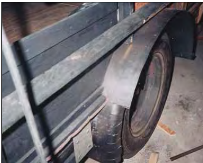
Cuts were made in the wheel wells to fit with the running boards.
