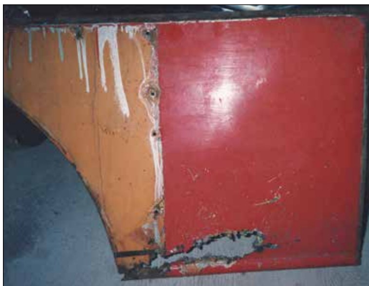
There was lot of rust to deal with. Here, a close-up of some of the damage the body had sustained.
