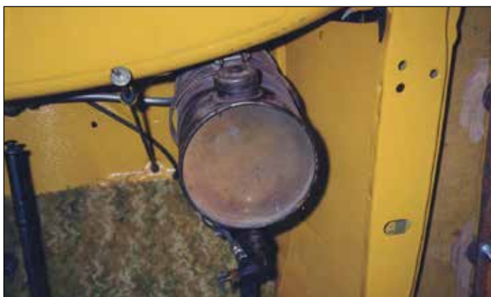
A small gas tank was added in case of emergencies.
