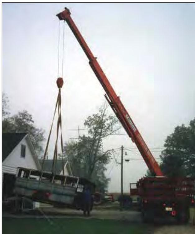
A crane lifts the bus body onto a trailer for transport to the Prenger garage.
